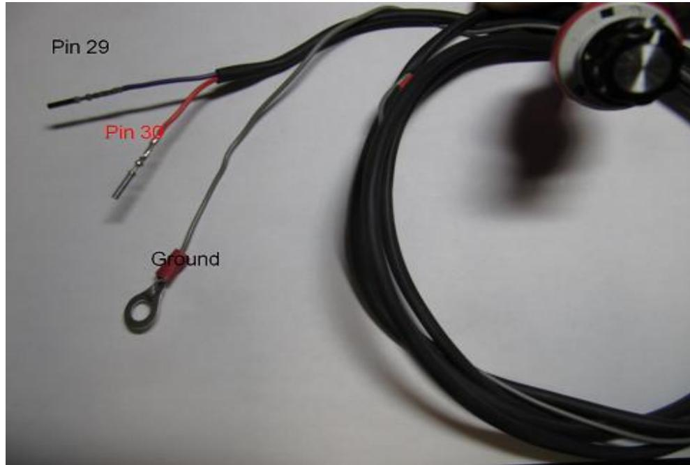
**Three wires out of the 4 stage switch. Two signals (29 and 30) and one ground**
